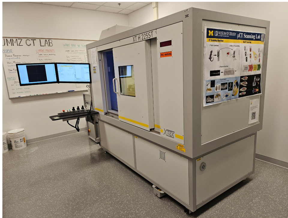
Figure 13. Micro computed tomography facility at the RMC.
