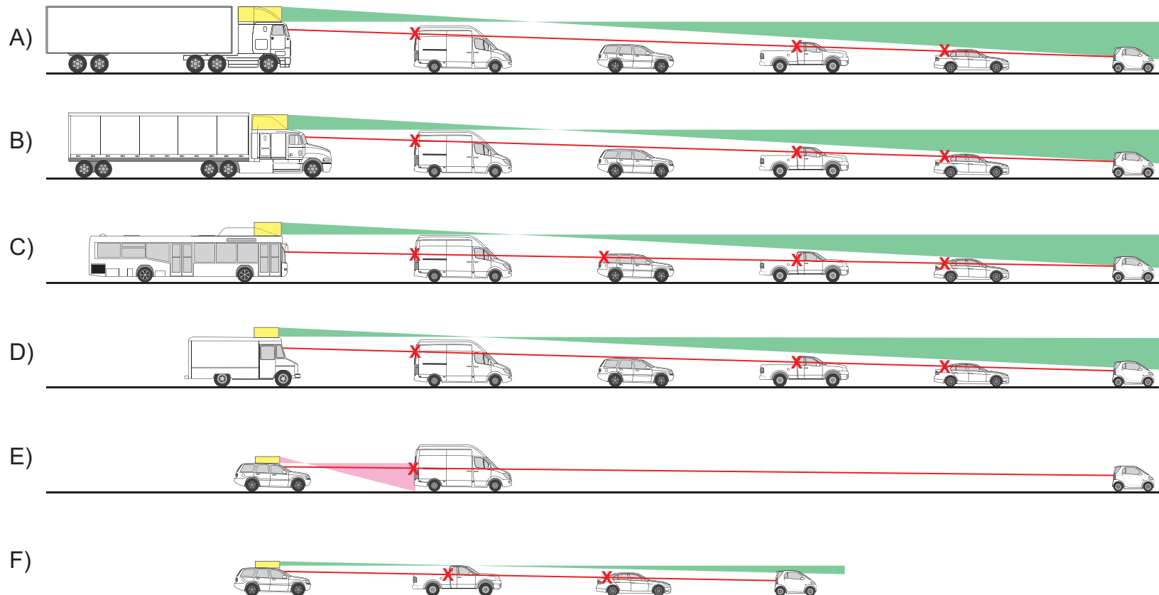
Figure 4. Example illustration (drawn to scale) of two heavy-duty vehicles and a bus (examples A through C), a medium-duty vehicle (example D), and a light-duty vehicle (examples E and F), and the corresponding vehicle geometries and lines of sight for direct driver vision and AV sensor coverage. (Distance from AV sensors to front vehicle: 50 m. Distance between vehicles: approximately 5 m [one car length]. The unobstructed AV sensor lines of sight shown in green do not correspond to the entire viewable area for the AV sensors but rather the applicable, unobstructed line of sight to traffic further ahead. This figure illustrates the ability of large trucks to see over light-duty vehicles, which constitute the majority of traffic on U.S. roads; it is unlikely that the AV sensors on a large truck would be able to see over another similarly large truck.)
