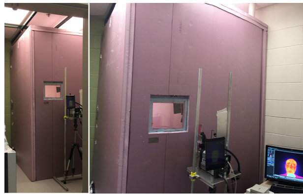
Figure 1: The experimental system including an insulating enclosure, physiological sensors, and thermal cameras.
